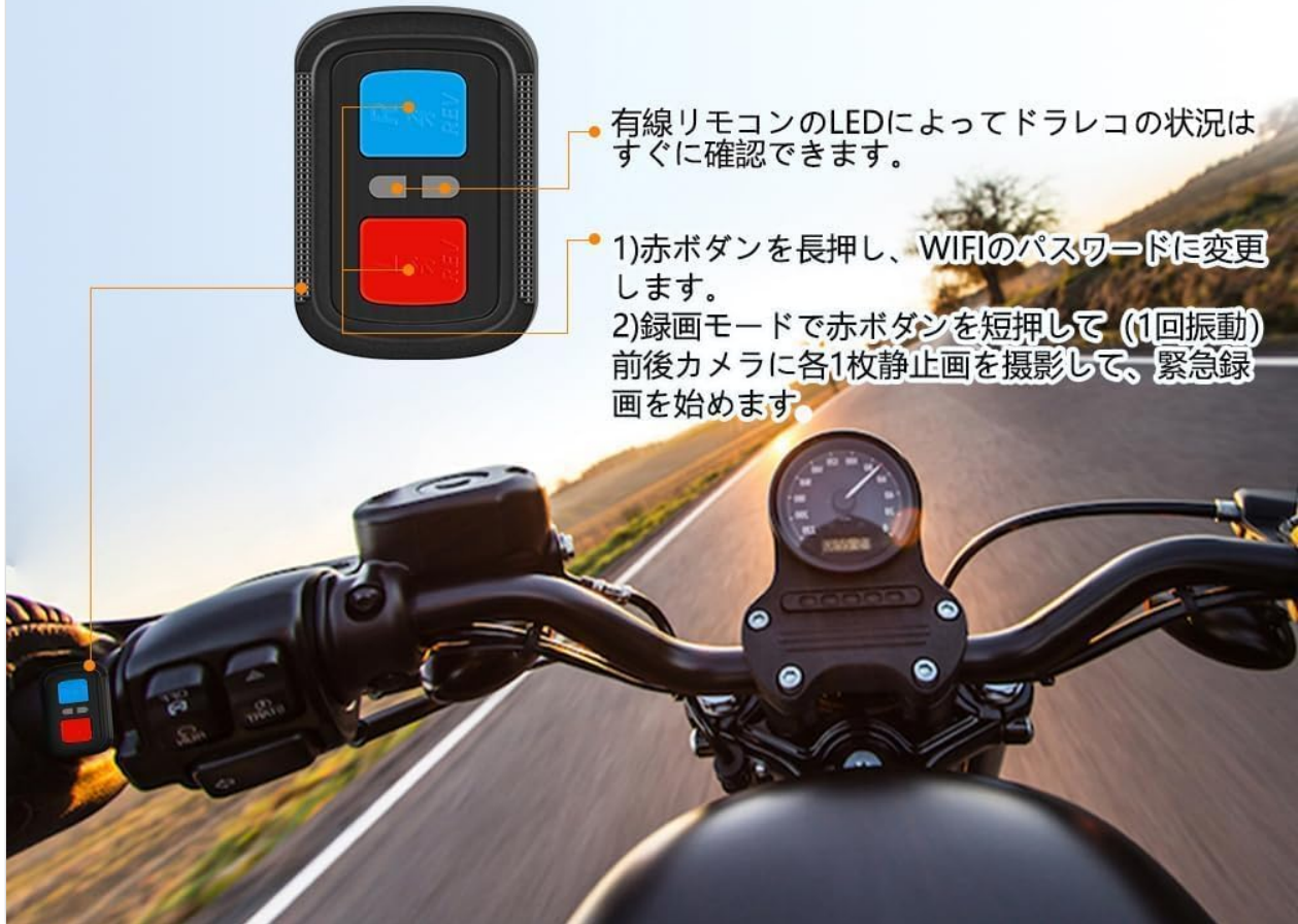
Figure 4.4: Wired remote control.
