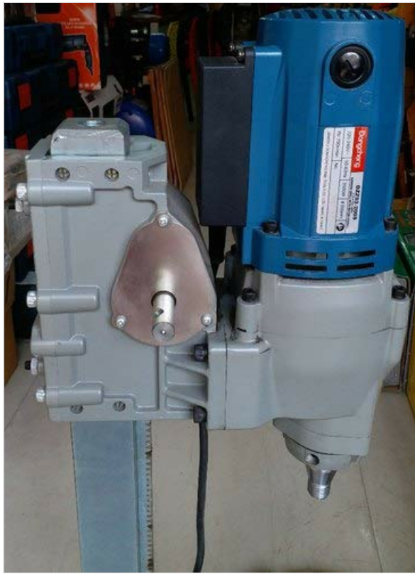
Figure 2.2: Detailed view of the drill motor unit and gearbox, highlighting the robust construction.
