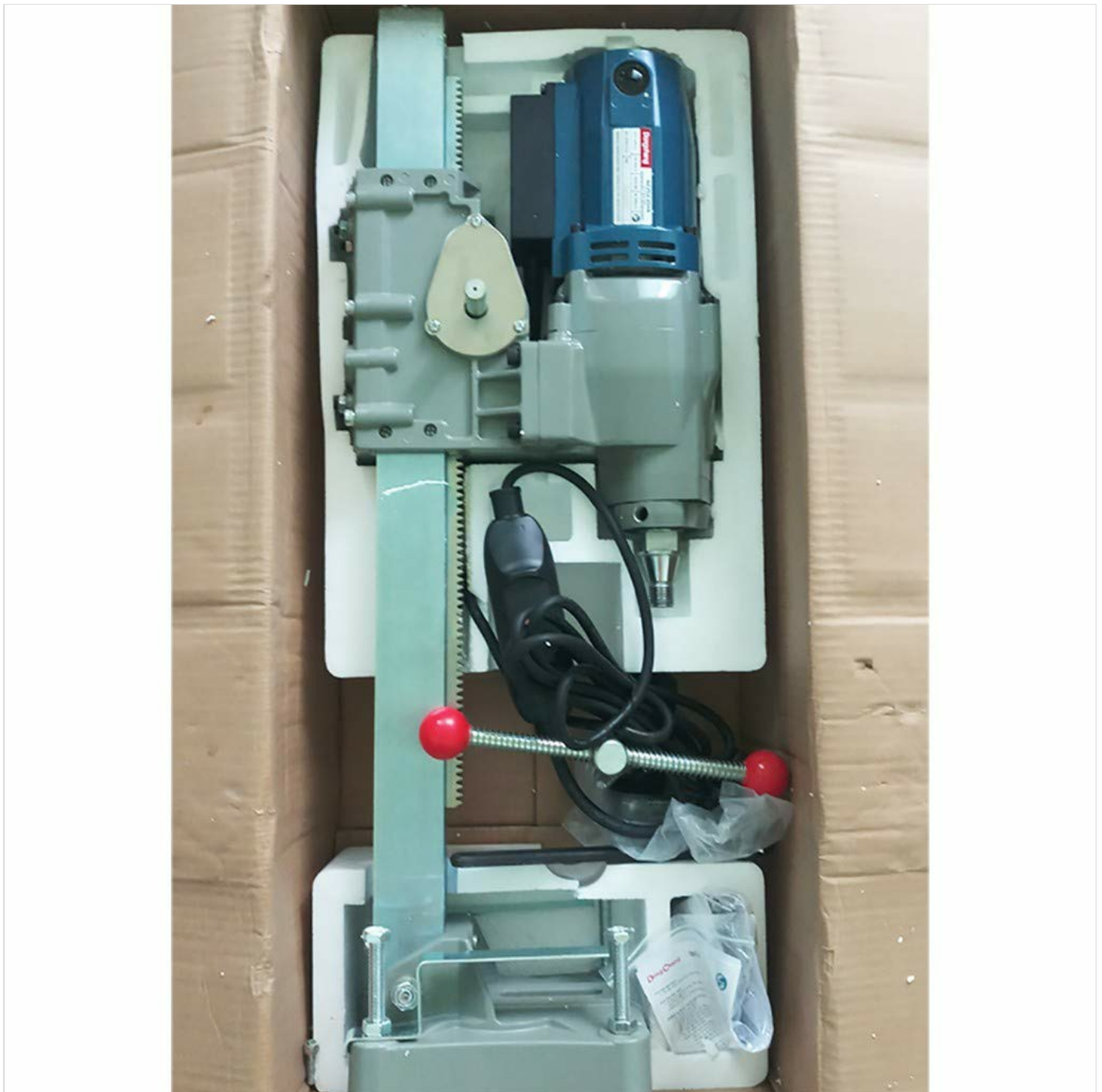
Figure 3.1: Components as received in packaging, including the drill motor, stand, and accessories.
