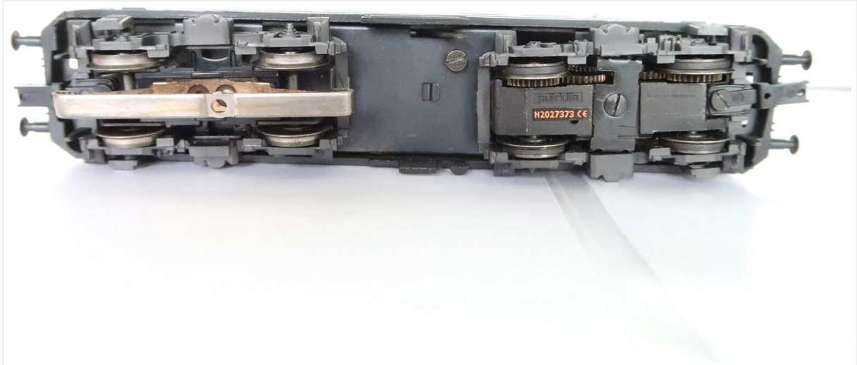
Figure 4.1: Underside view of the locomotive, highlighting the wheel sets and the central pickup shoe essential for power collection on Marklin 3-rail systems.
