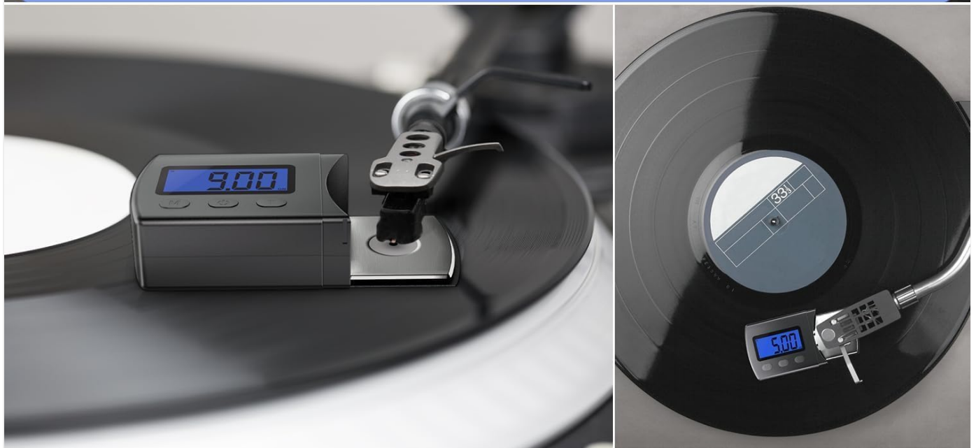
Image: A composite image demonstrating the stylus force gauge in action on various turntables, highlighting its role in accurately setting tracking force for optimal vinyl playback and cartridge longevity.
