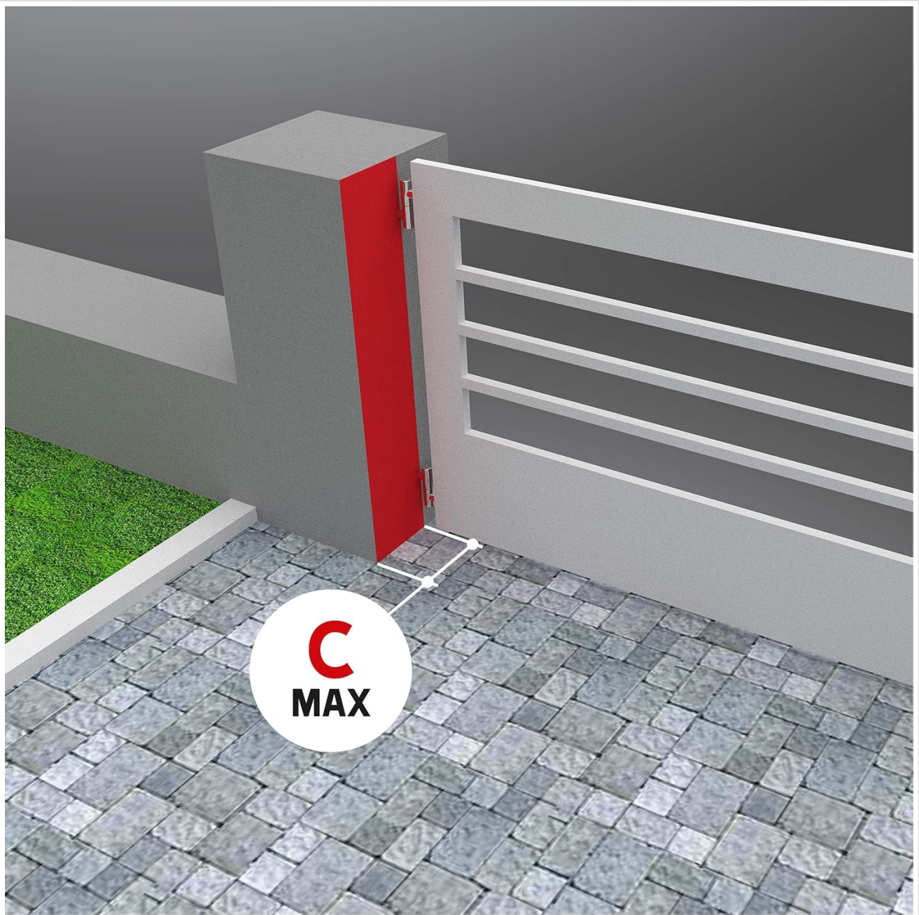
Image: An illustration showing the 'C' dimension, which is the critical distance from the gate hinge to the motor's mounting bracket. This measurement must be within the specified limits for proper gate operation.
