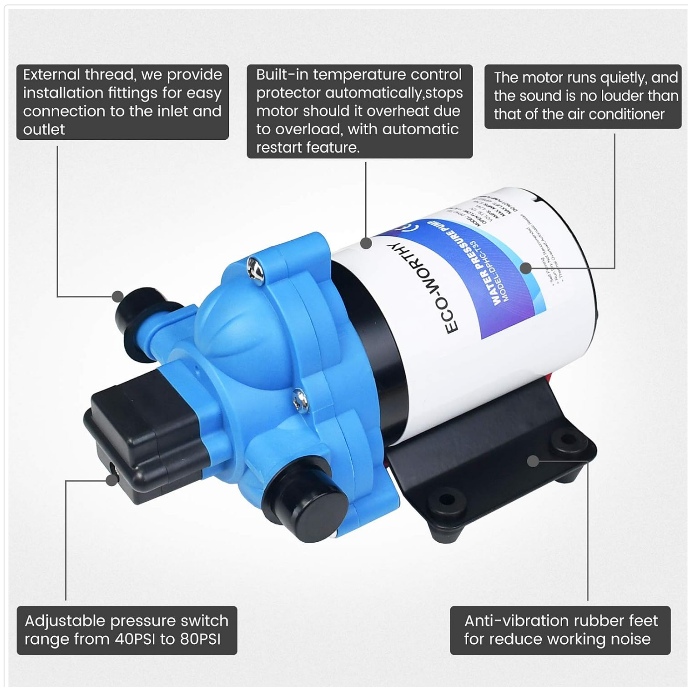
Image: Detailed view of the pump highlighting key features: external thread fittings for inlet/outlet, built-in temperature control protector, quiet motor, adjustable pressure switch (40-80 PSI), and anti-vibration rubber feet.
