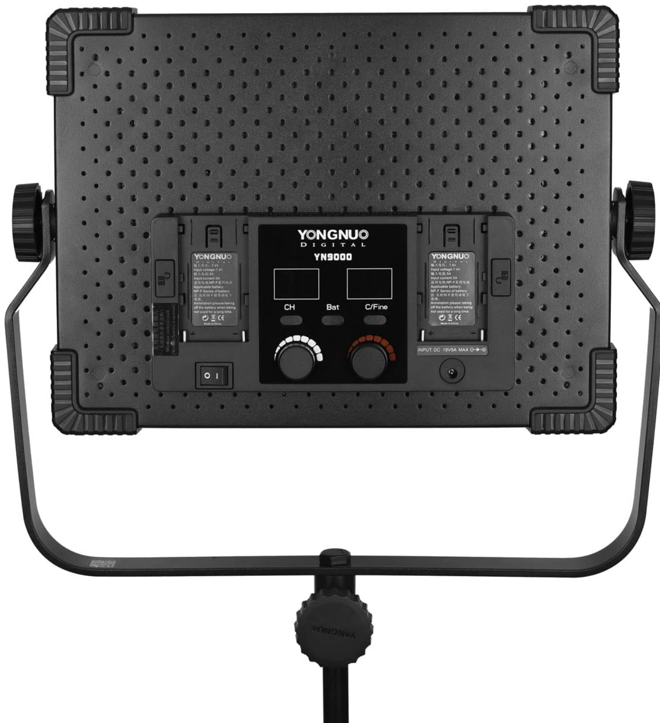
Image 2.2: Rear panel of the YONGNUO YN9000 LED Video Light. This image highlights the control interface, including the power switch, channel (CH) and battery (Bat) indicators, fine-tuning (C/Fine) knob, and two NP-F battery slots, along with the DC power input.
