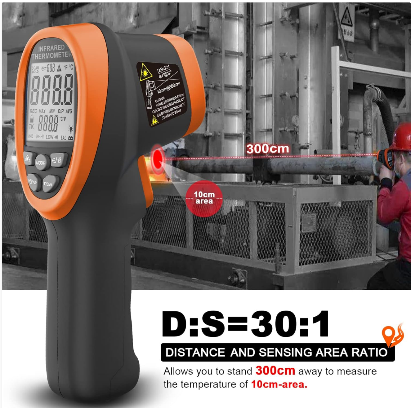
Figure 6.2: Explanation of the 30:1 D:S ratio, showing how distance affects the measurement spot size.
