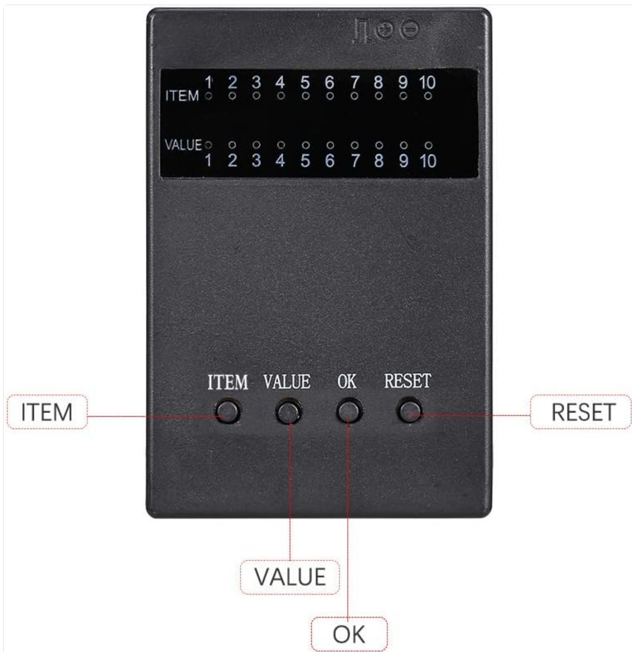
Image: Close-up view of the GoolRC Programming Card, highlighting the ITEM, VALUE, OK, and RESET buttons.
