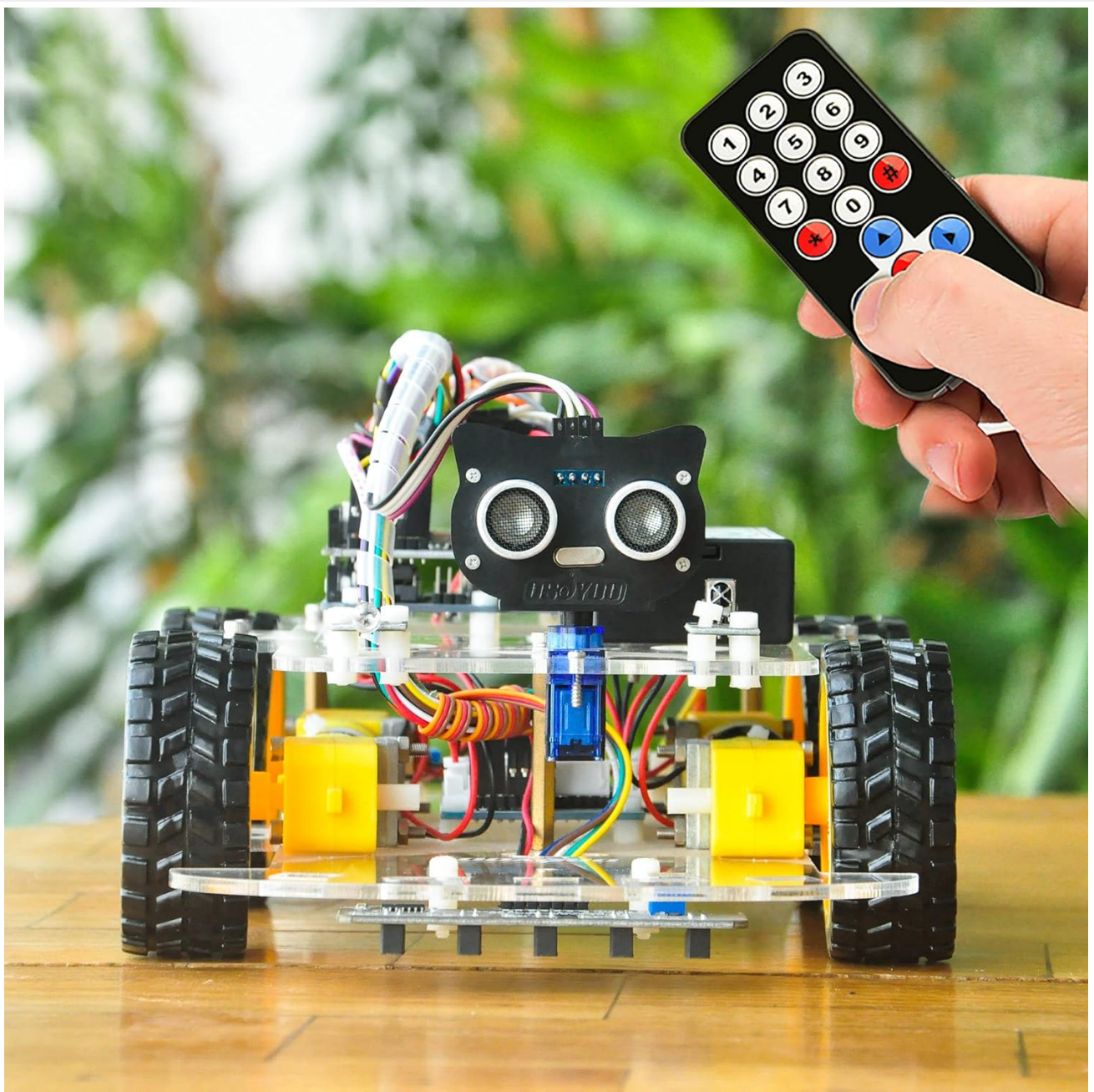
Figure 3: Operating the robot car with the IR remote control.
