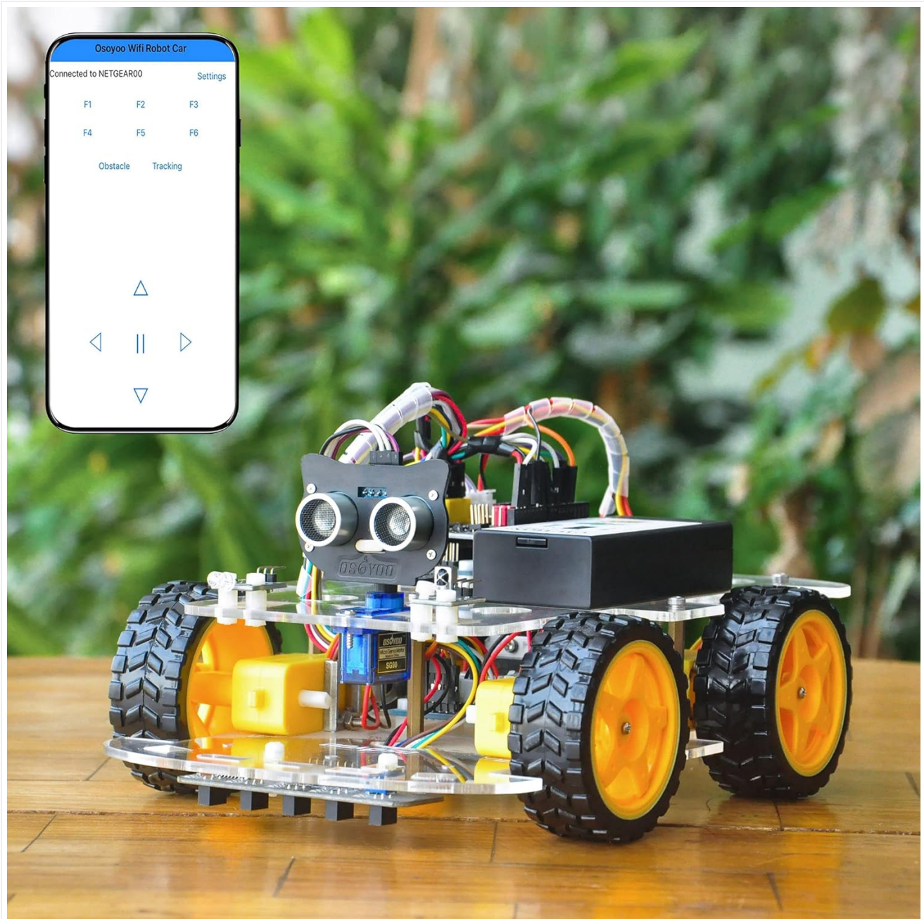
Figure 2: Controlling the robot car via a smartphone app.
