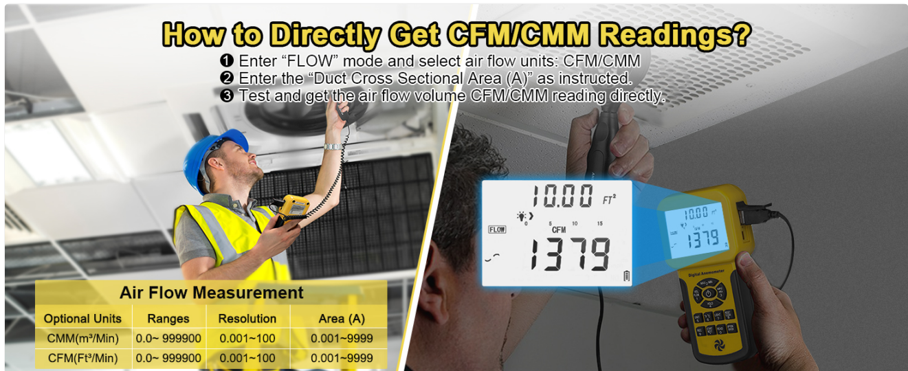
Figure 6.2: Visual guide on how to obtain direct CFM/CMM readings using the AIOMEST AI-856A, including steps for entering flow mode, selecting units, and inputting the duct cross-sectional area.
