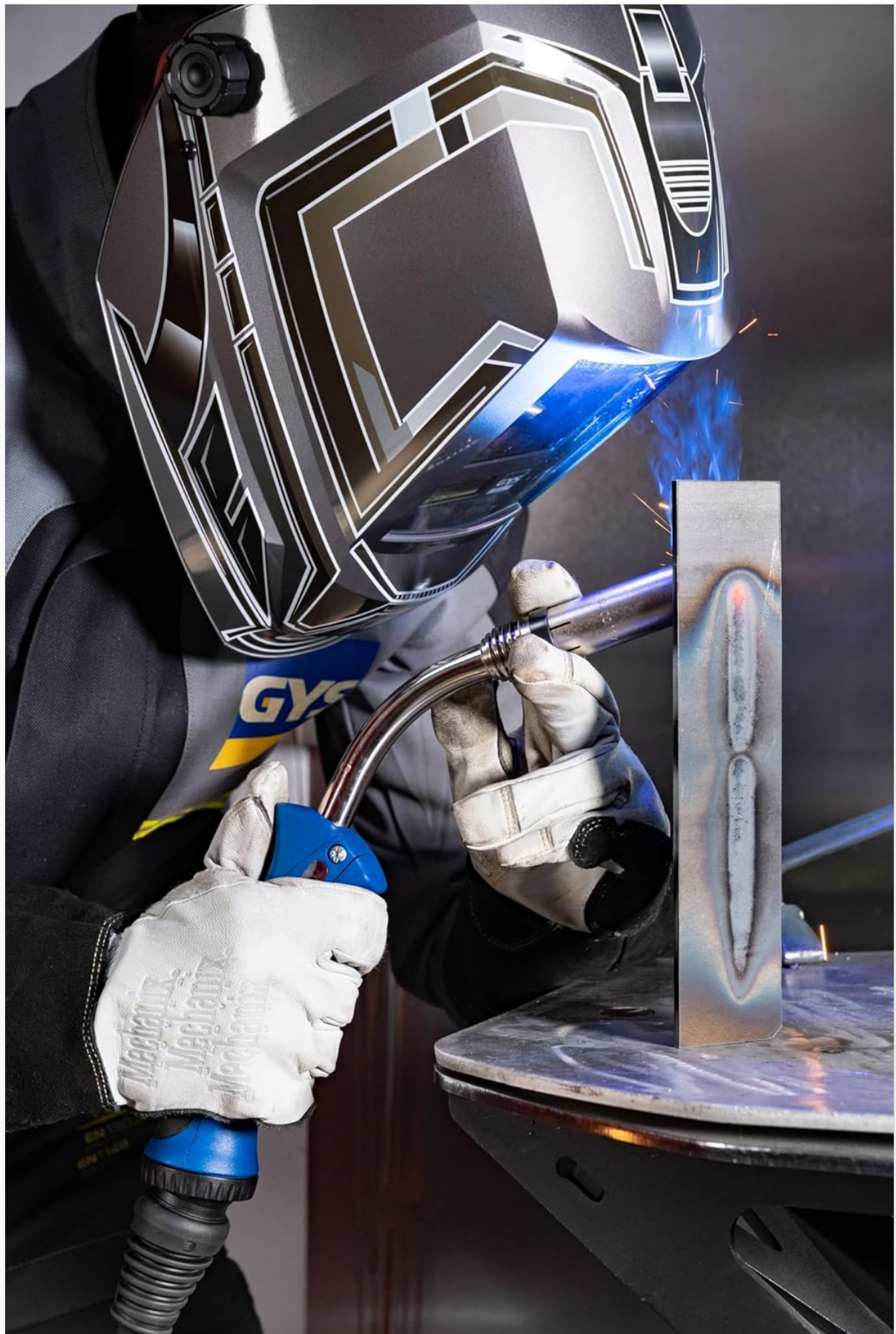
Image 5.1: A welder demonstrating the use of a MIG/MAG torch on a metal workpiece, wearing appropriate safety gear.
