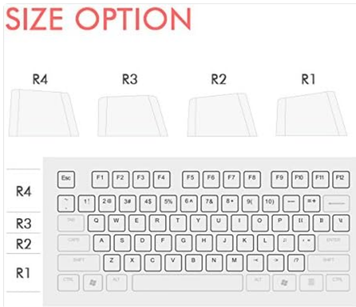
Figure 2: Diagram illustrating the different keycap profiles (R1, R2, R3, R4) and their typical placement on a standard mechanical keyboard layout. This helps in selecting the correct keycap for a specific row.
