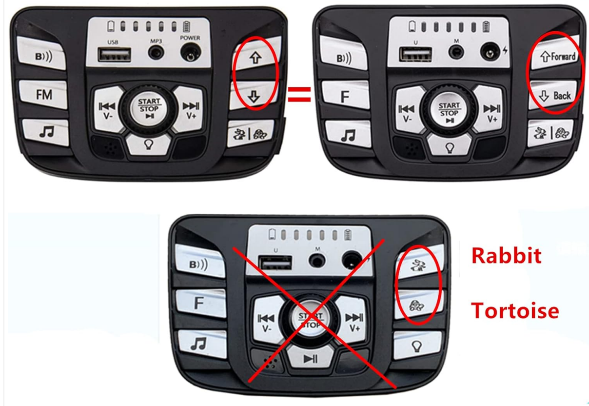
Figure 4: Comparison of panel types, highlighting variations in speed control buttons.
