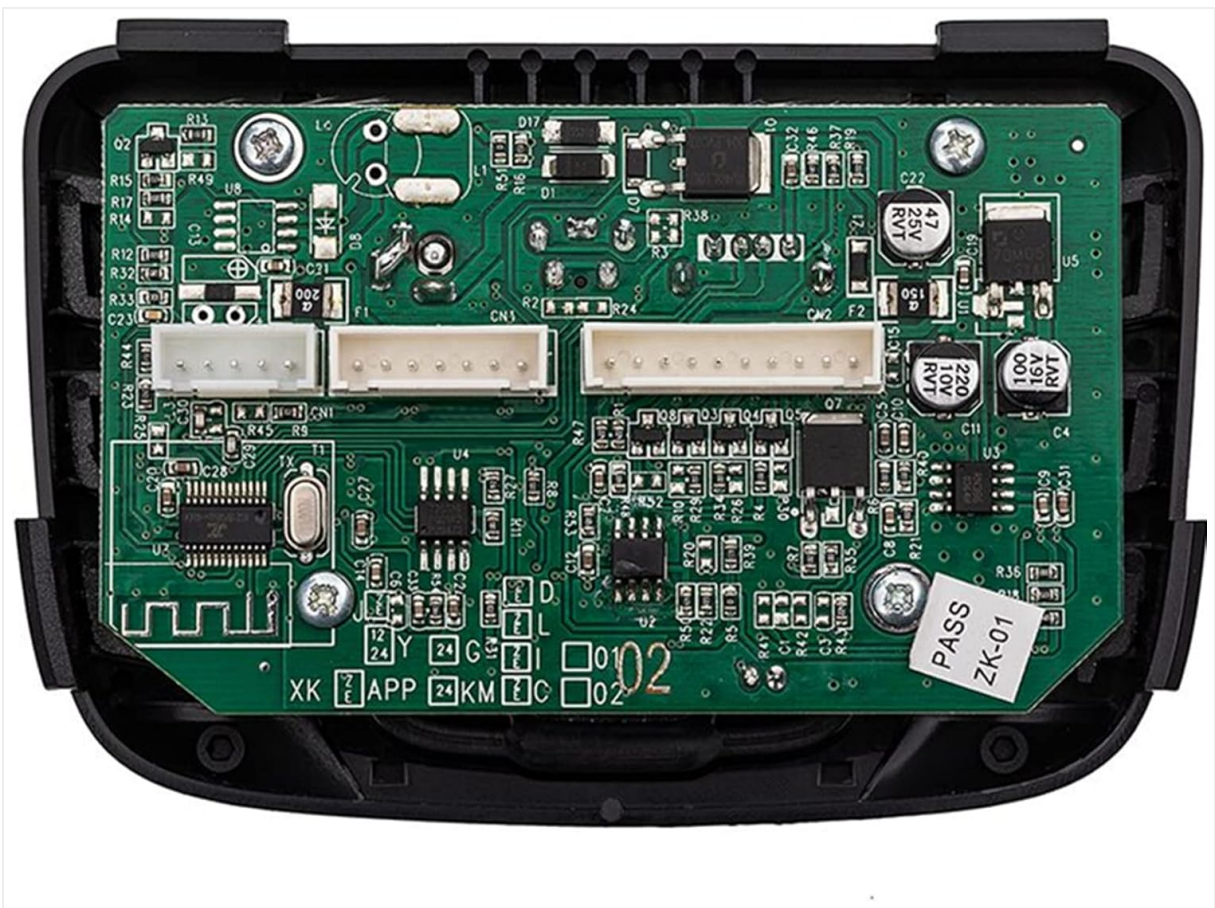
Figure 2: Rear view of the PCB, illustrating various connection points for wiring harnesses.
