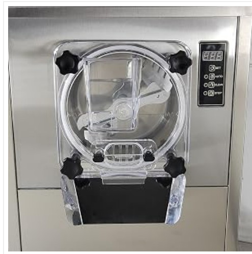
Figure 3.3: Internal view of the freezing cylinder, highlighting the 360-degree rotation of the agitator for thorough mixing and freezing.
