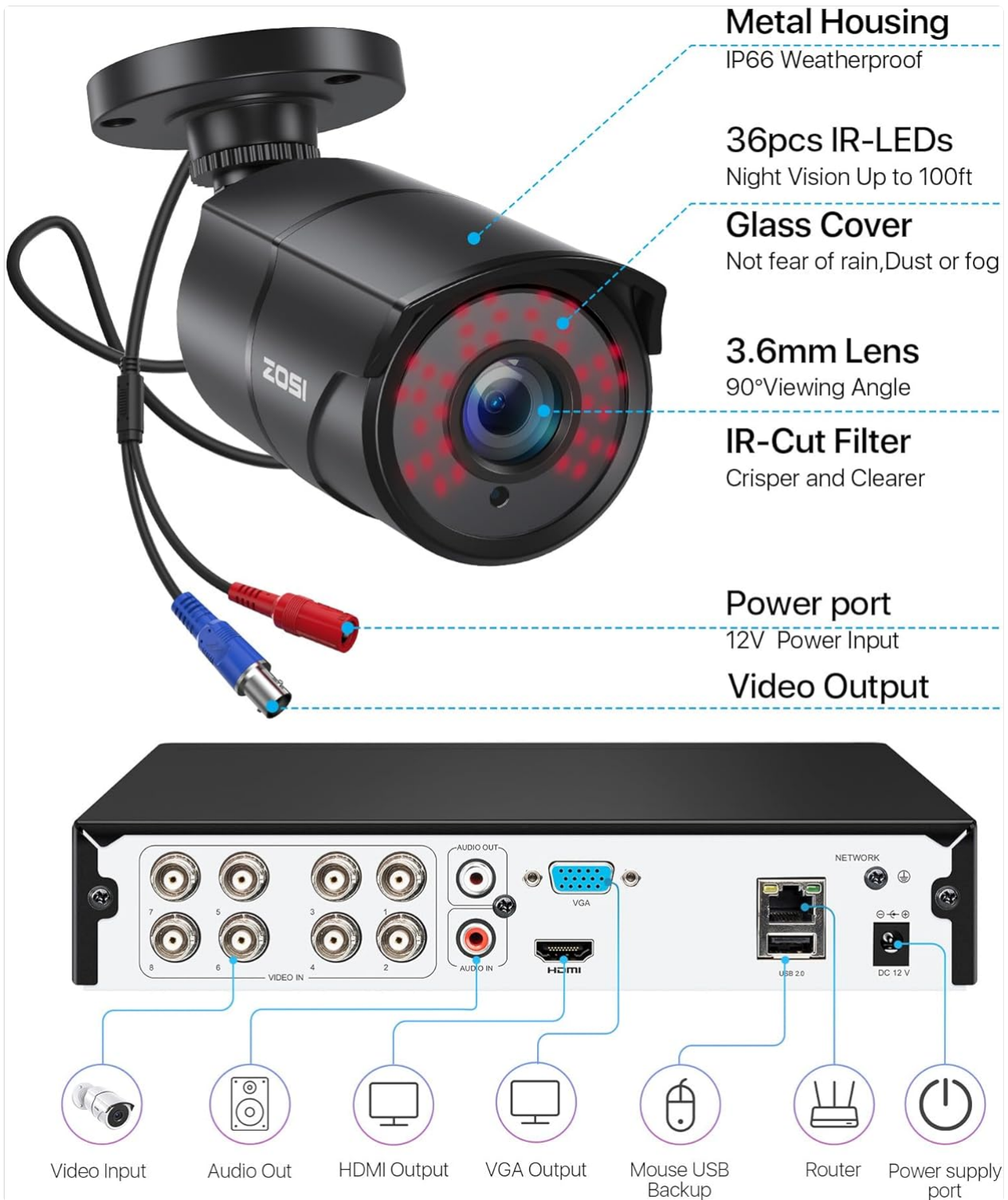
Figure 3.2: Detailed view of camera features and DVR connection ports.
