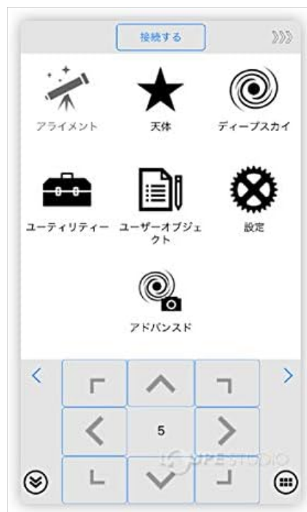
Figure 6: Main menu of the SynScan Pro app. This image illustrates the various functions available in the app, including alignment, celestial object selection, deep sky objects, utilities, user objects, settings, and advanced options.
