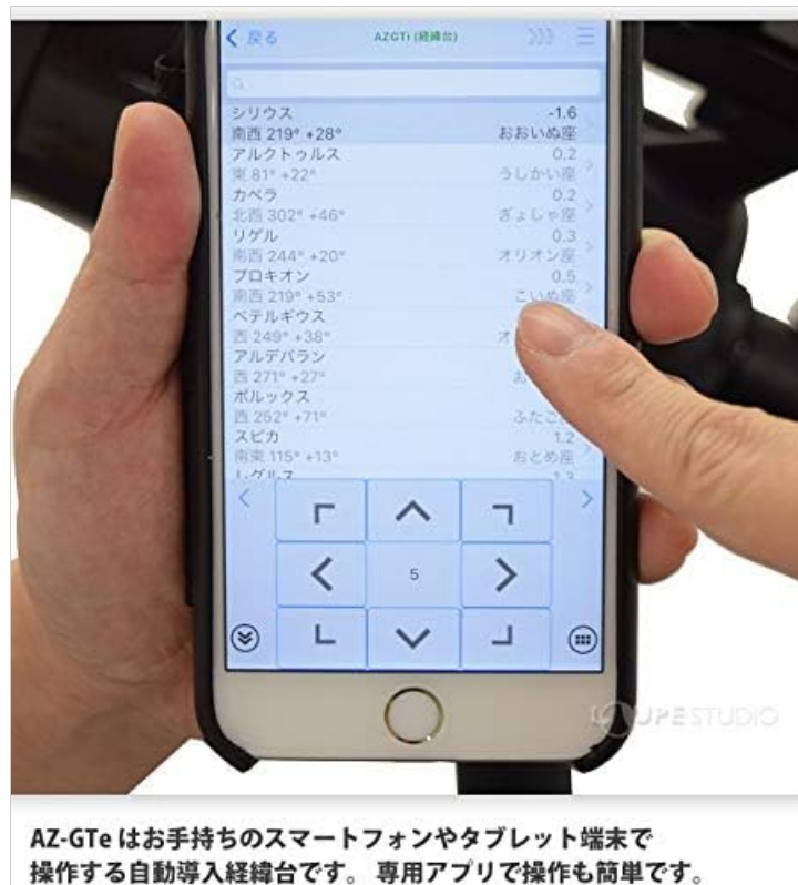
Figure 5: Smartphone app interface for object selection and control. This image shows the SynScan Pro app displaying a list of celestial objects and directional control buttons for precise telescope movement.
