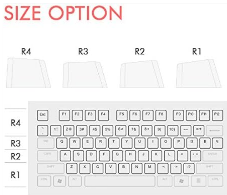
Figure 2: Keycap Size Options and Typical Keyboard Placement.
