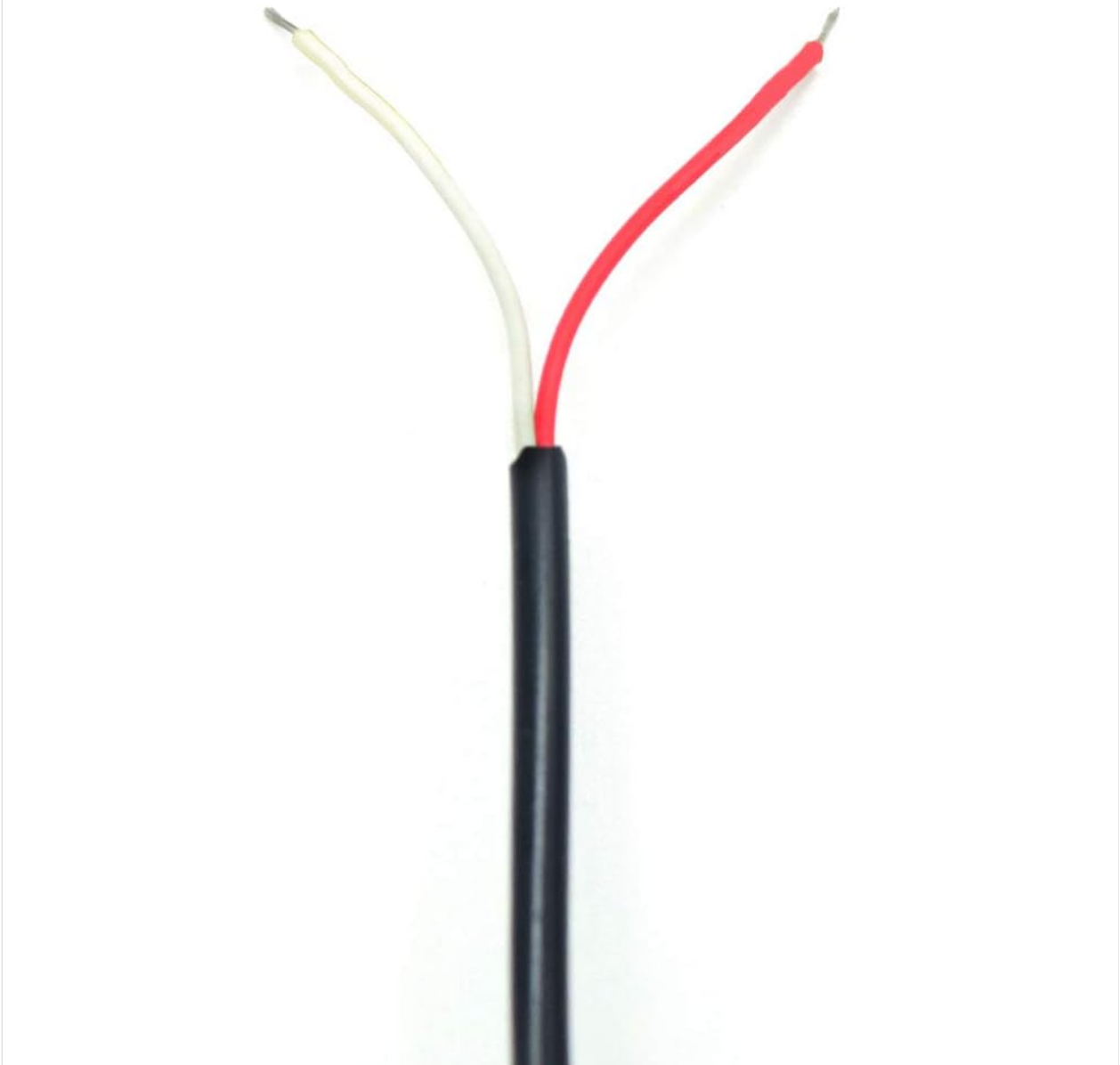
Image: Close-up of the red (ACC/Battery+) and white (GND/Battery-) input wires.
