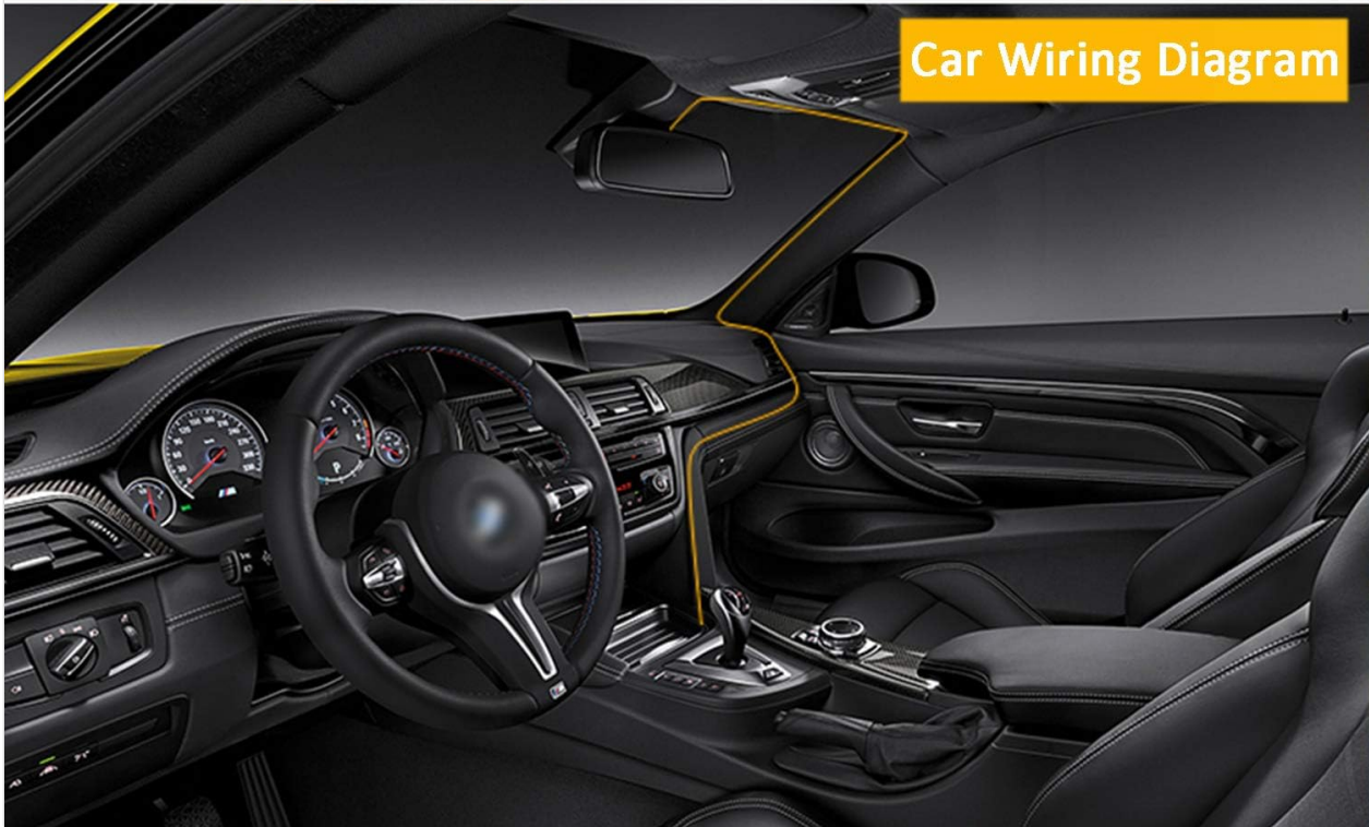
Image: Illustrative diagram of a car interior with suggested cable routing for a dash cam hardwire kit.
