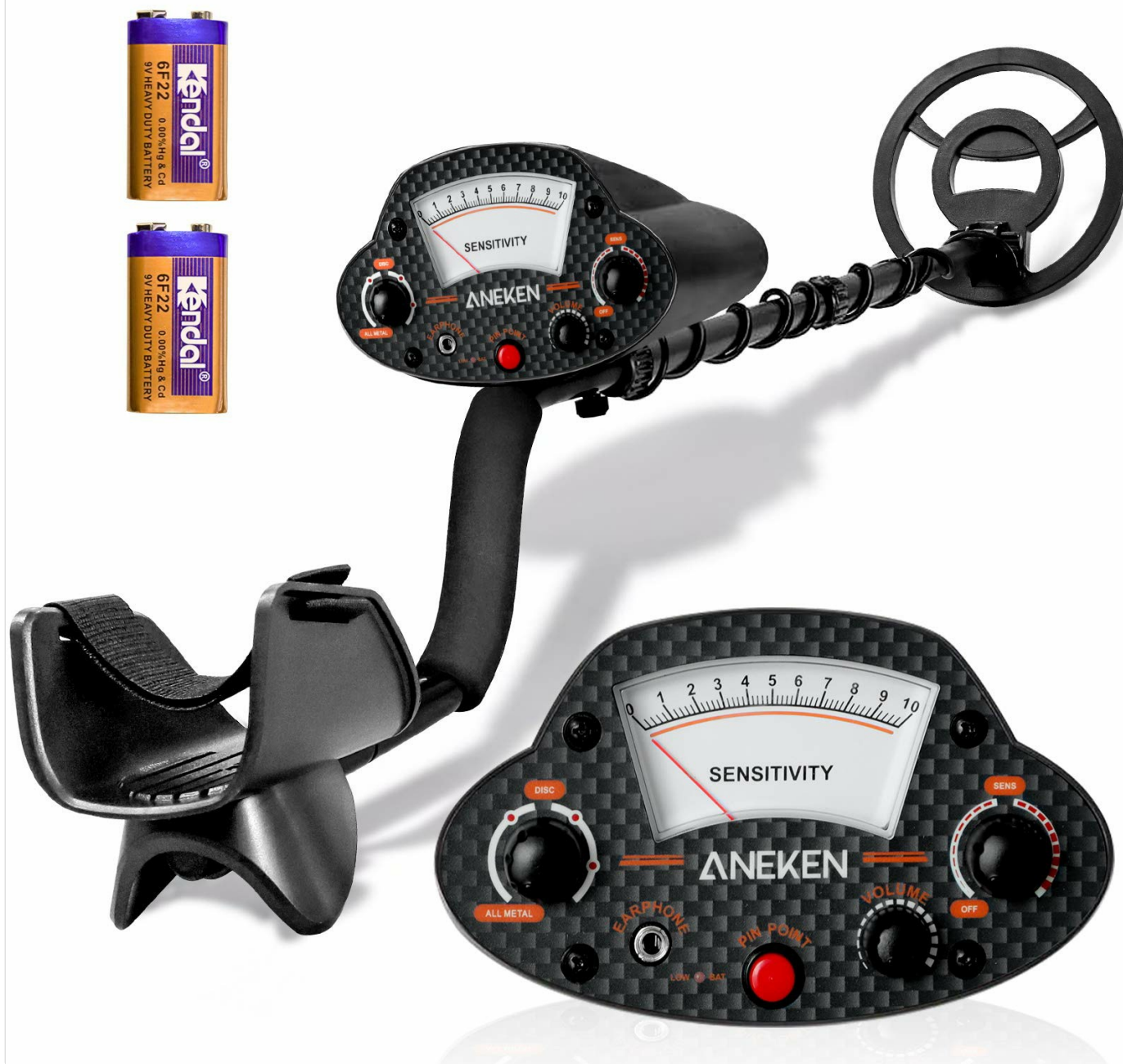
Image: Close-up of the Aneken MD-5050 control panel, showing the sensitivity dial, volume control, DISC knob, pinpoint button, and headphone jack. This image highlights the main operational controls.
