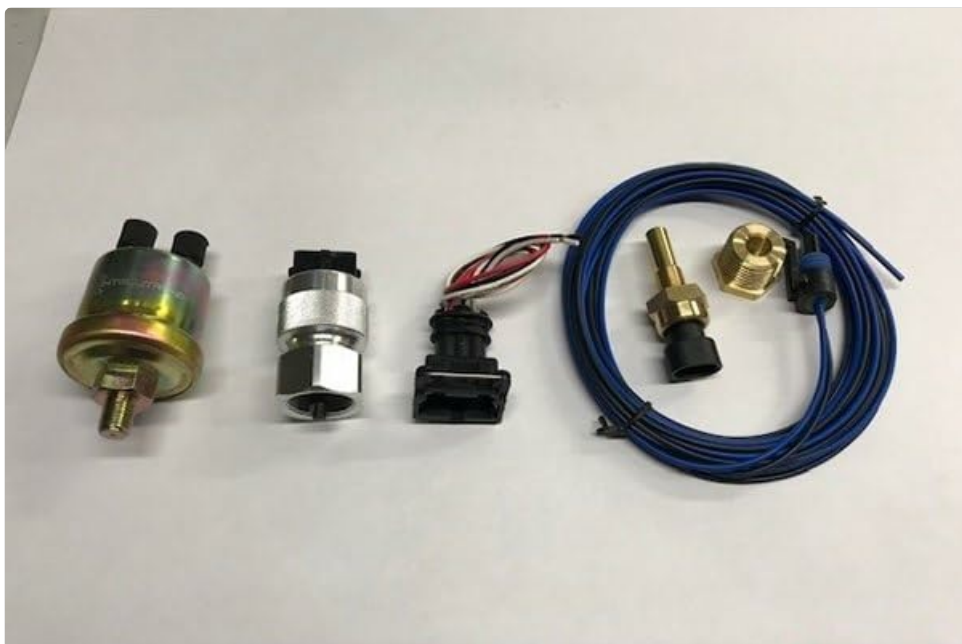
Image 2.2: Close-up of the included sending units, typically for oil pressure and water temperature, which are essential for the digital gauges to function.
