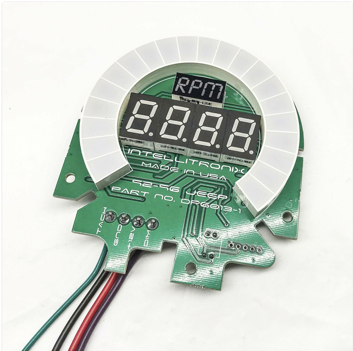
Image 4.2: Detailed view of the RPM gauge circuit board, indicating connections for power and signal input.
