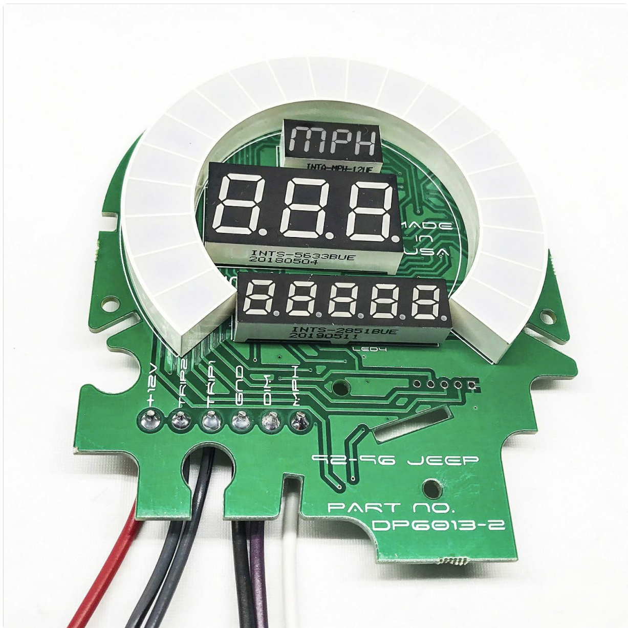
Image 4.3: Detailed view of the MPH gauge circuit board, showing connections for speed sensor input and power.
