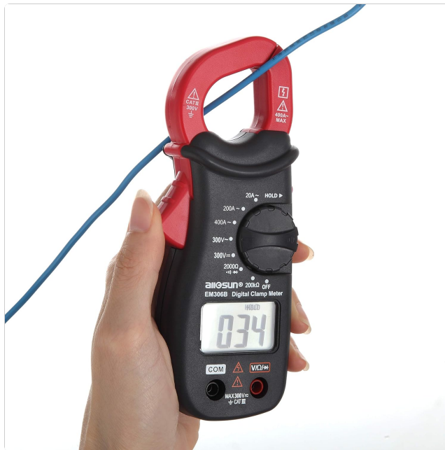
Image: A hand demonstrating how to use the clamp meter to measure current on a single electrical wire.
