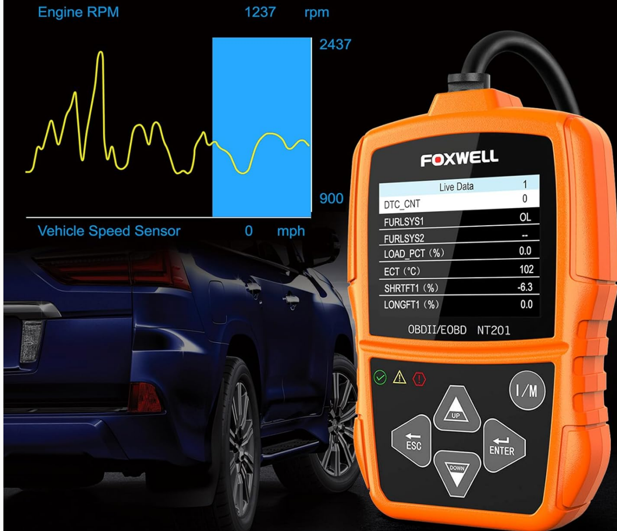
Image 4.3: The NT201 showing real-time vehicle sensor data in both text and graph formats.
