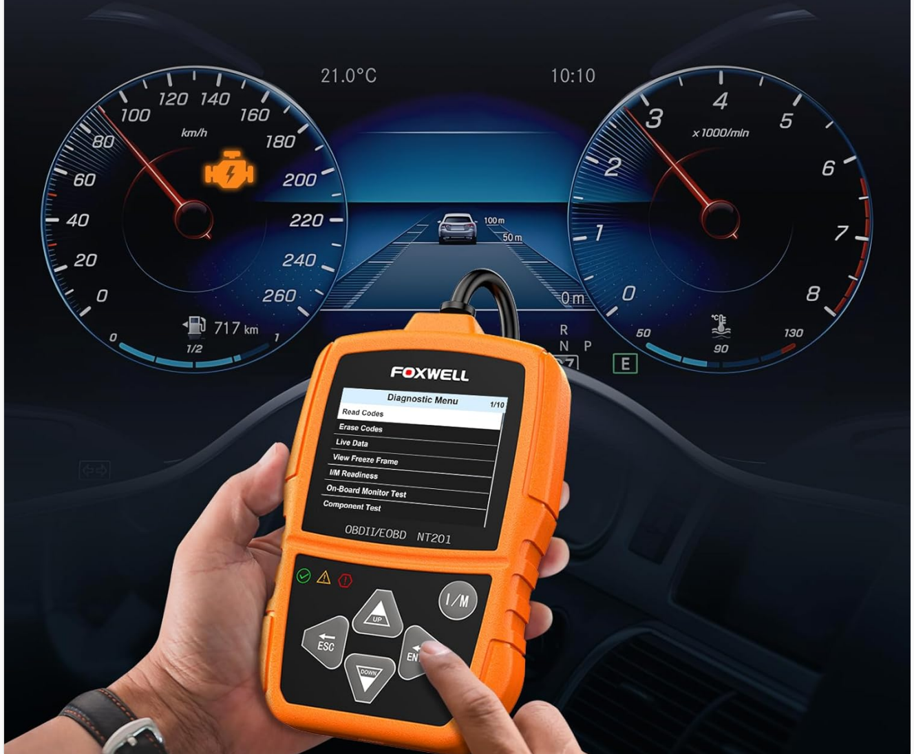
Image 4.1: The NT201 scanner in use, showing the process of checking the engine light.
