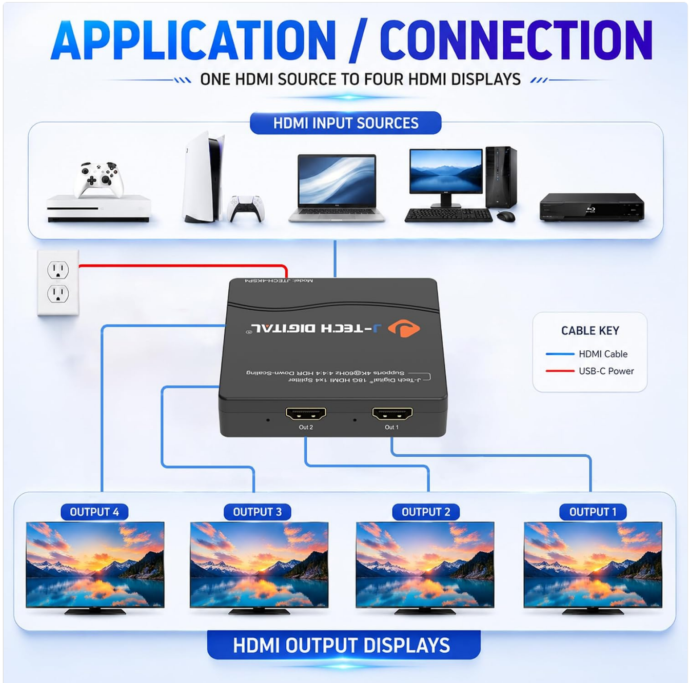
Image 5.1: Application and connection diagram for the JTECH-4KSP4 HDMI Splitter. This visual guide demonstrates how to connect one HDMI input source (such as a gaming console, laptop, or PC) to the splitter, and then connect the splitter's four outputs to individual HDMI displays.
