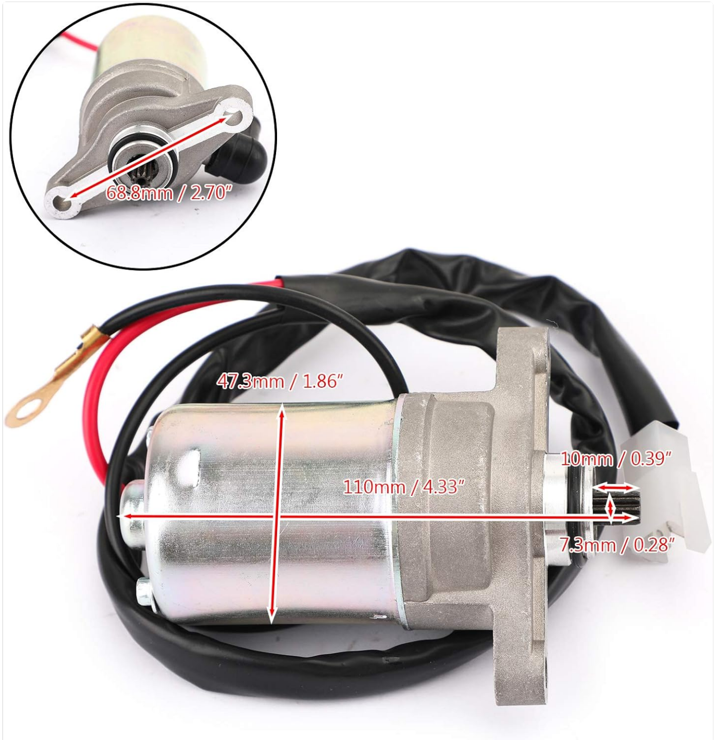
Image: Artudatech Starter Motor with key dimensions highlighted. The image shows the overall length of 110mm (4.33"), a width of 47.3mm (1.86"), gear OD of 7.3mm (0.28"), and a 10mm (0.39") shaft diameter.
