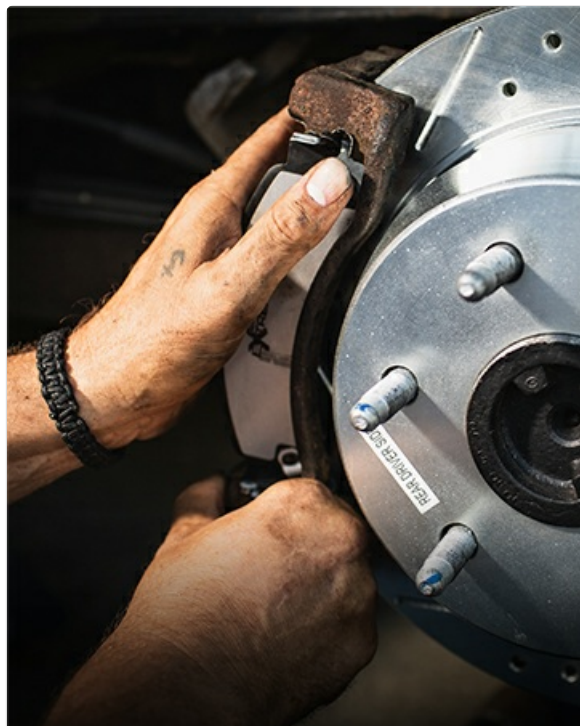
Image 4.1: A close-up view of a mechanic's hands installing a new brake pad into a caliper assembly. This illustrates a critical step in the brake pad replacement process, emphasizing the need for careful handling and proper seating of components.
