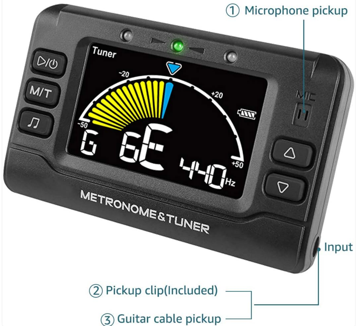
Figure 3: The three ways to pick up sound: built-in microphone, clip-on pickup, and direct guitar cable input.
