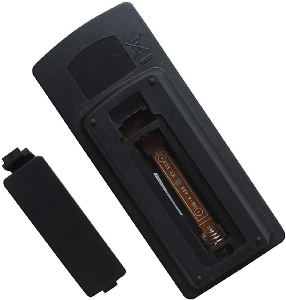
Figure 2: Back of the remote control with the battery compartment open, illustrating correct AAA battery insertion.
