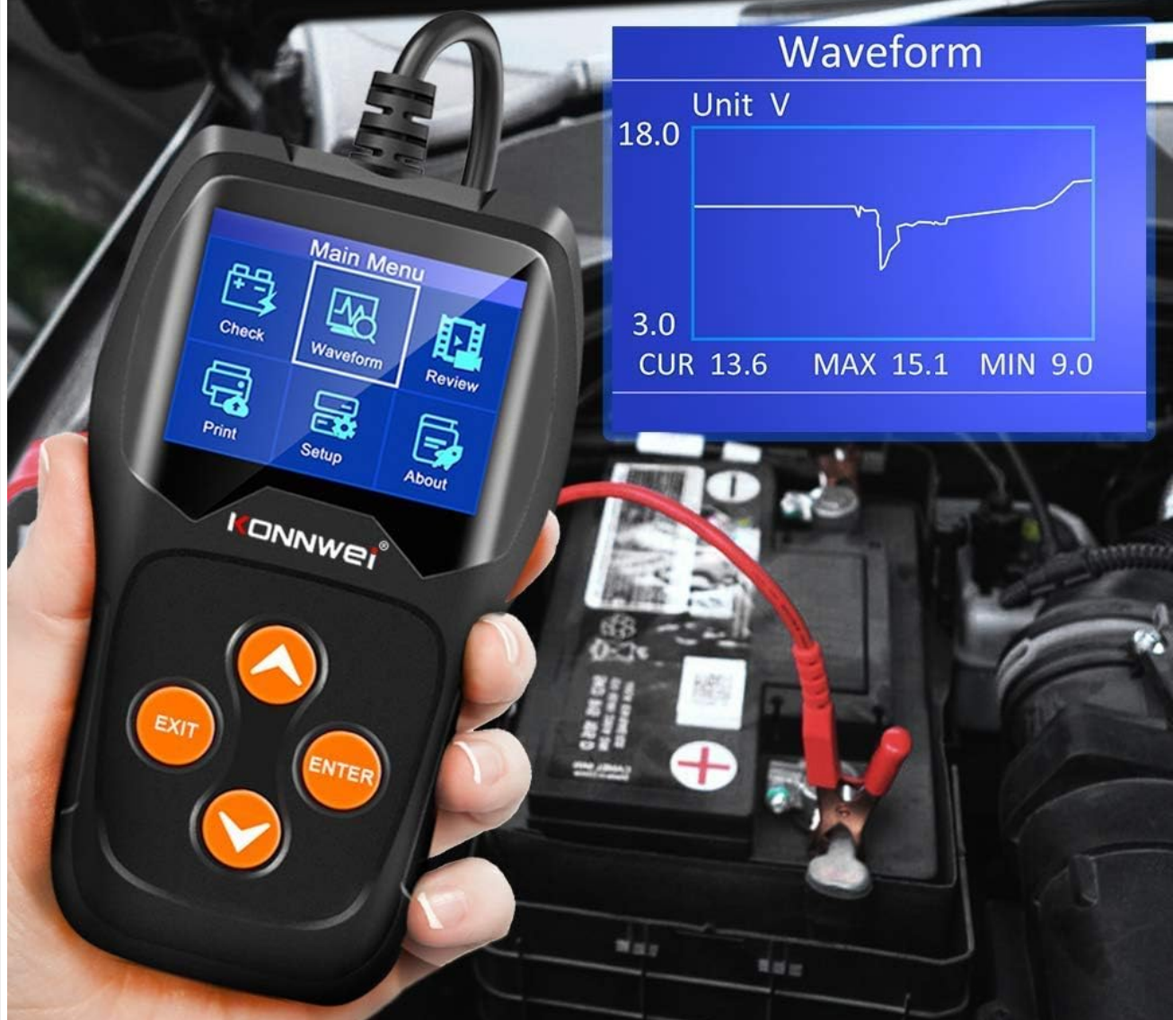
Image 2.4: The KW600's waveform graphing function, illustrating voltage changes over time for diagnostic purposes.
