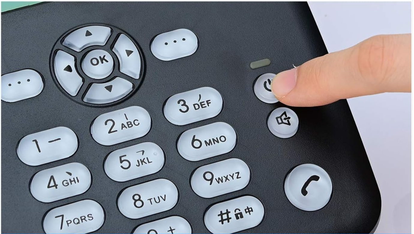
Step3: Press the red power button, the deskphone will turn on
