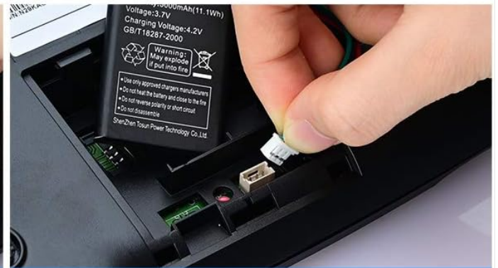
Step2 : Insert the battery (included)
