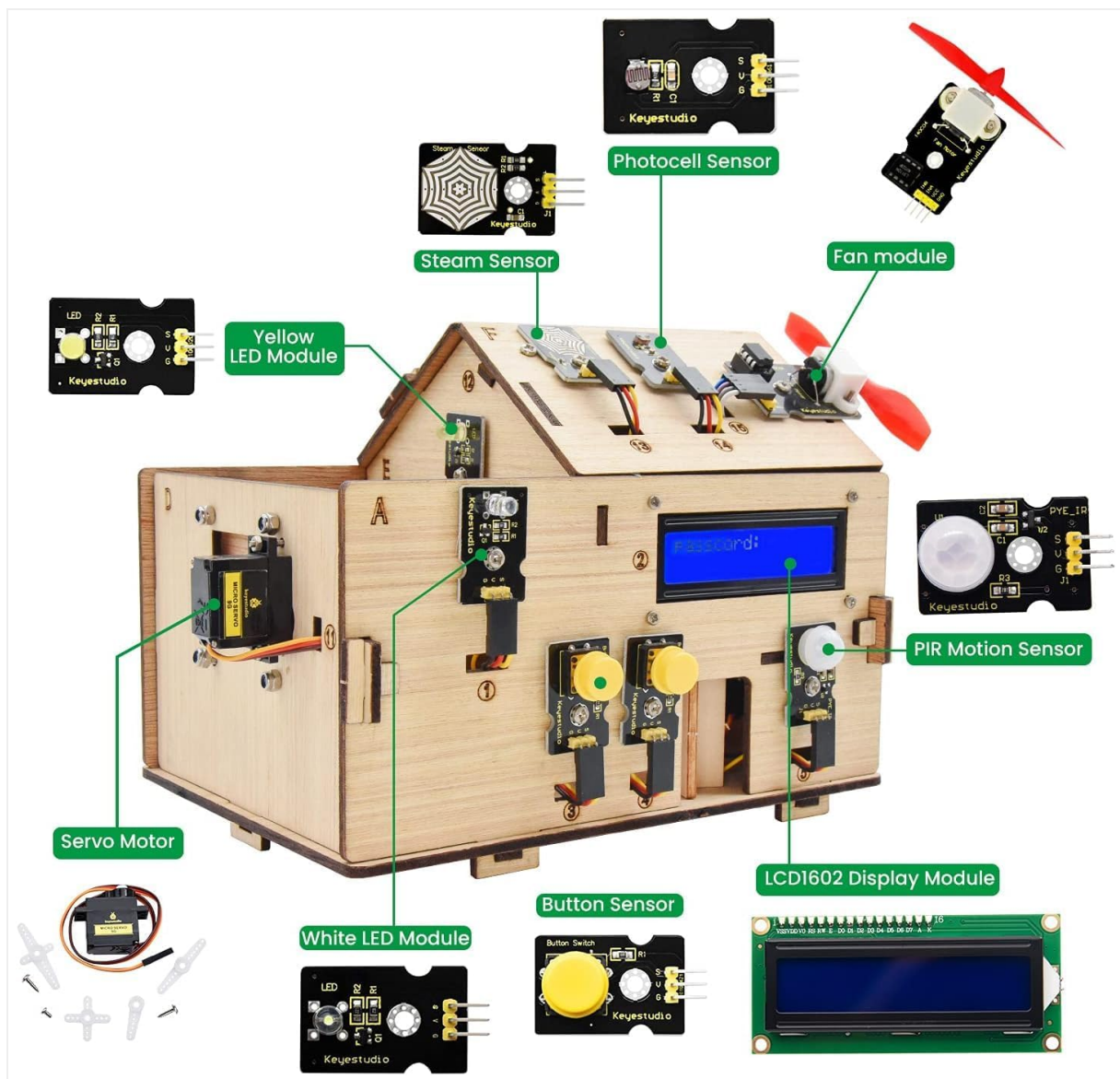
Figure 2.2: Assembled smart home model with key sensors and modules labeled, including photocell, steam sensor, fan module, yellow LED, PIR motion sensor, servo motor, white LED, button sensor, and LCD1602 display.
