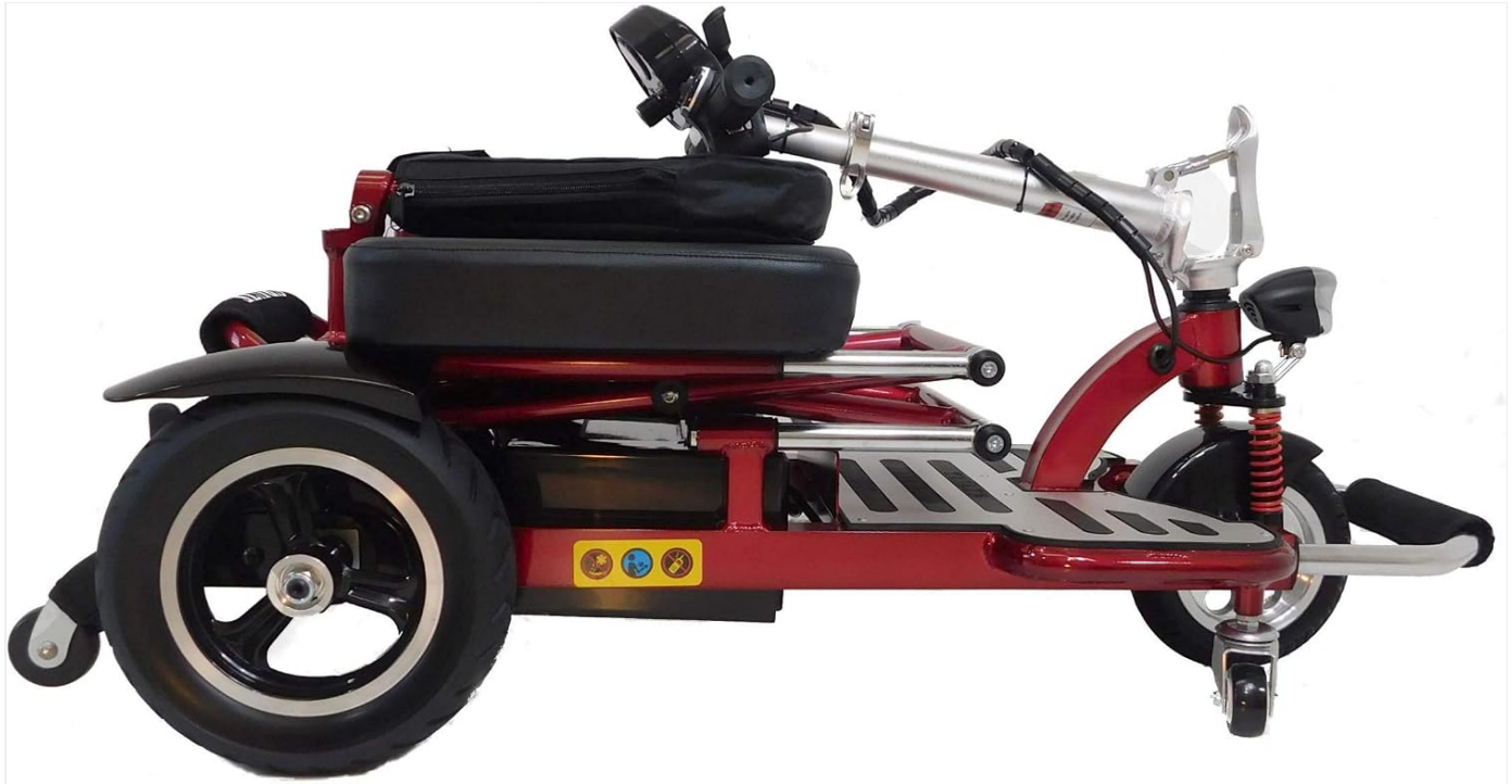
Figure 2: The TRIAXE Cruze Mobility Scooter in its folded configuration. Note: This image shows a red scooter, but the folding mechanism is identical for the blue model.
