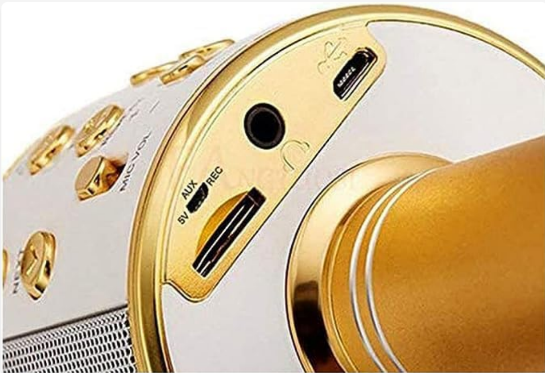
Figure 3.1: Close-up view of the microphone's charging (USB) and audio (AUX) ports.
