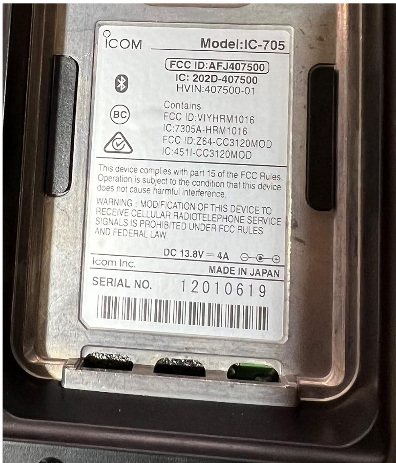
Figure 5: FCC Label and Serial Number. This label provides regulatory information and the unique serial number of the unit.
