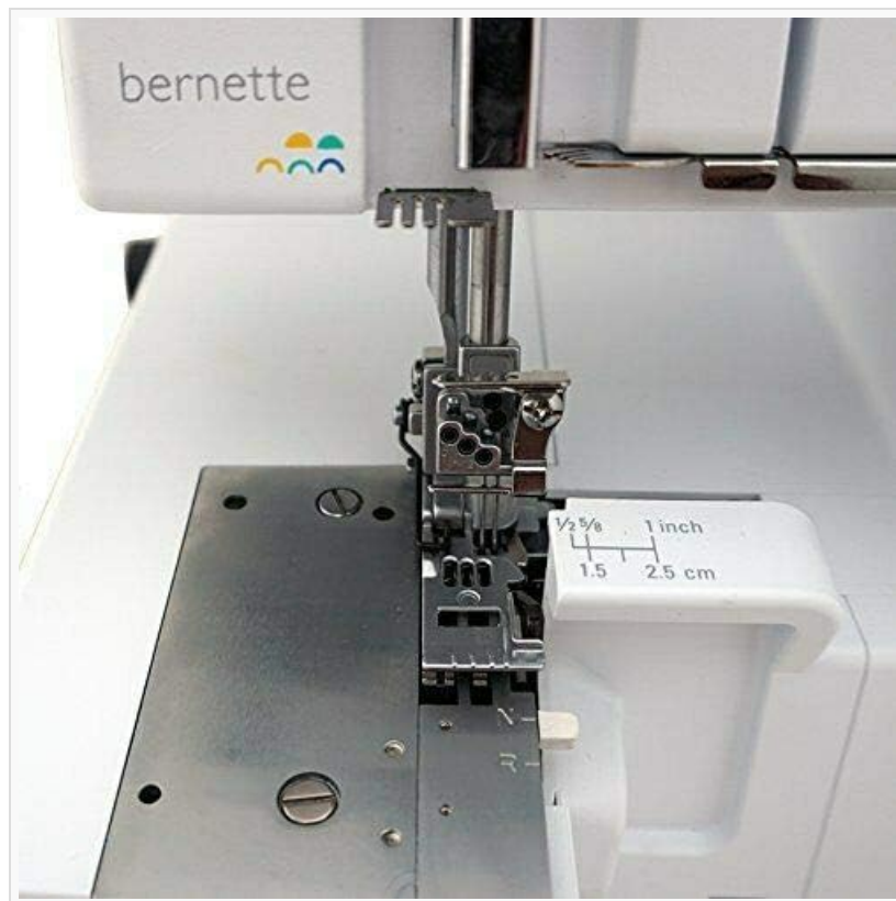
Figure 3.2: Detailed view of the needle area, presser foot, and stitch plate, indicating measurement markings.
