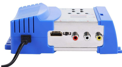
Figure 2.7: Side view of the modulator, clearly showing the HDMI input port and the Audio/Video (RCA) input ports for connecting source devices.
