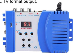
Figure 2.5: Visual representation of the modulator's flexible output channel options, supporting both NTSC and PAL TV formats for broad compatibility.
