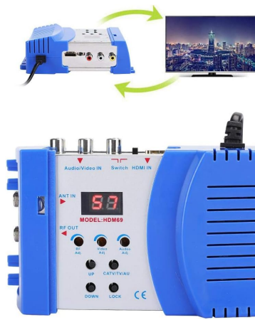
Figure 2.2: Connection diagram illustrating the modulator's role in converting signals for TV display. The image shows the modulator with arrows pointing to a television screen, indicating signal transmission.
