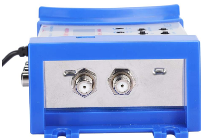
Figure 2.8: Opposite side view of the modulator, displaying the RF IN and RF OUT coaxial ports for antenna connection and signal distribution.
