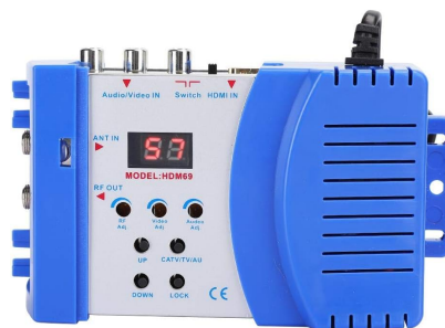
Figure 2.1: Front view of the RF Modulator, displaying the digital channel indicator, model number (HDM69), and controls for RF, Video, Audio adjustment, and channel selection (UP/DOWN/CATV/TV/AU/LOCK).
