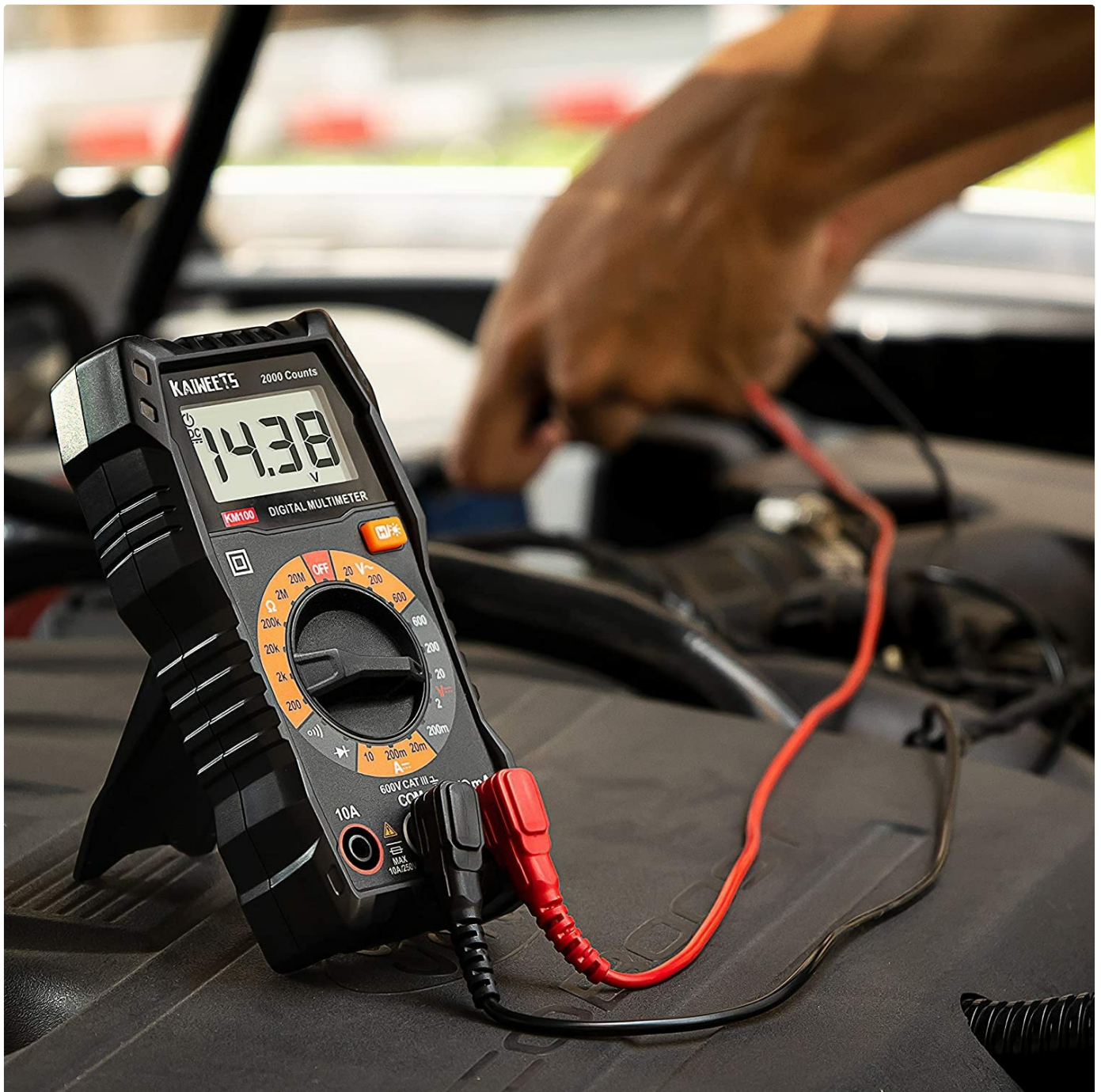
Figure 5: Measuring DC Voltage on a car battery.
