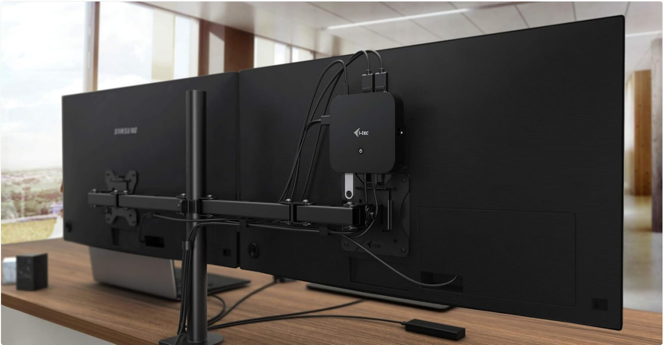
Image 5.2: Docking station mounted behind a VESA compatible monitor for a clean desk setup.
