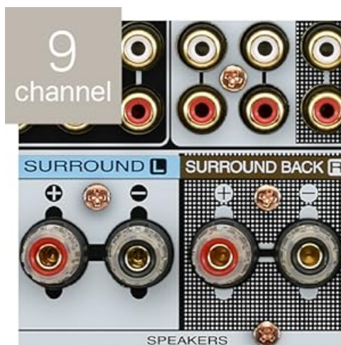
Close-up image showing the clearly labeled 9-channel speaker terminals on the Marantz SR7015.
