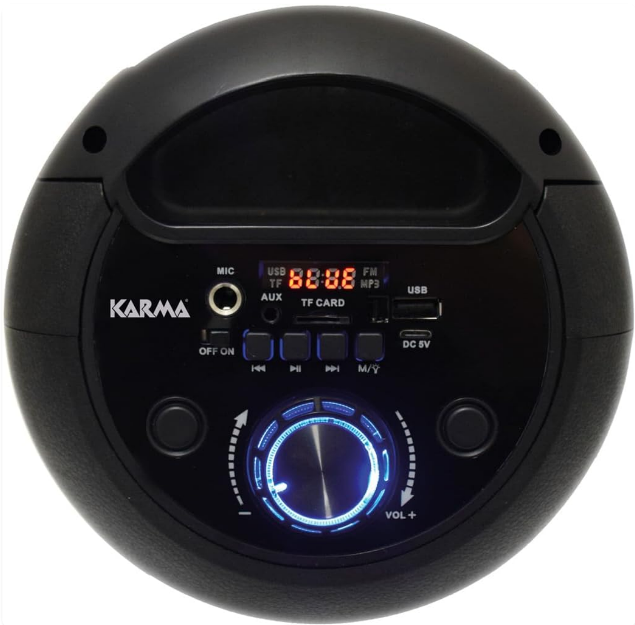
Image 1: Close-up view of the Karma HPS T252R speaker's control panel, showing various ports and buttons including USB, TF card slot, AUX input, microphone input, power switch, mode button, playback controls, and volume knob.
