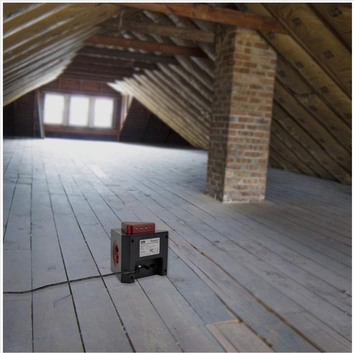
Figure 3: Example placement of the device in an attic for optimal coverage.
