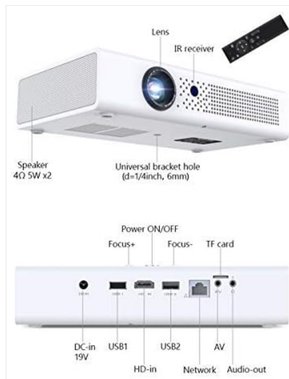
Image 4.1: Diagram illustrating the projector's components and ports.
