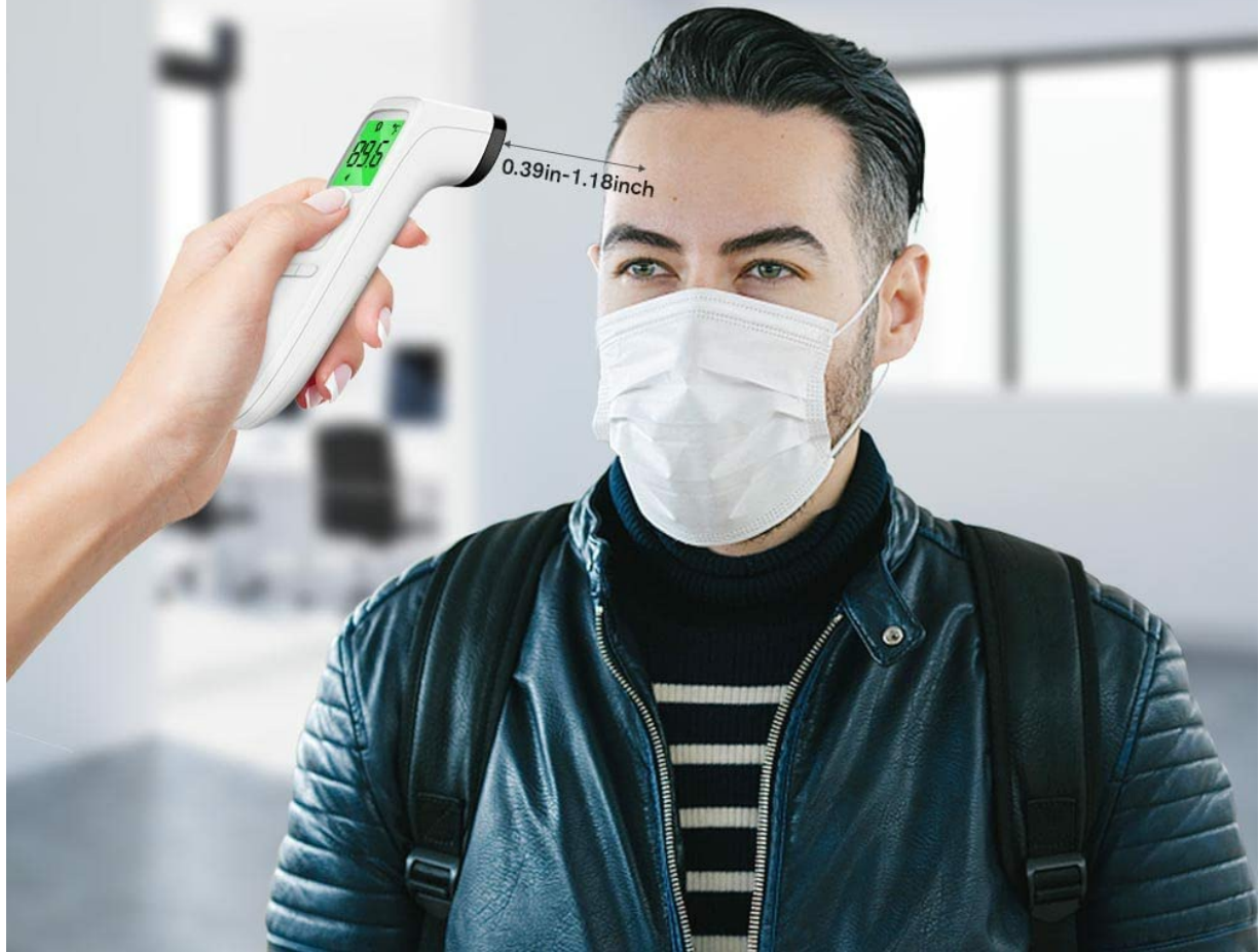
Figure 3: Demonstrates the non-contact measurement system, showing the correct distance for taking a forehead temperature.
