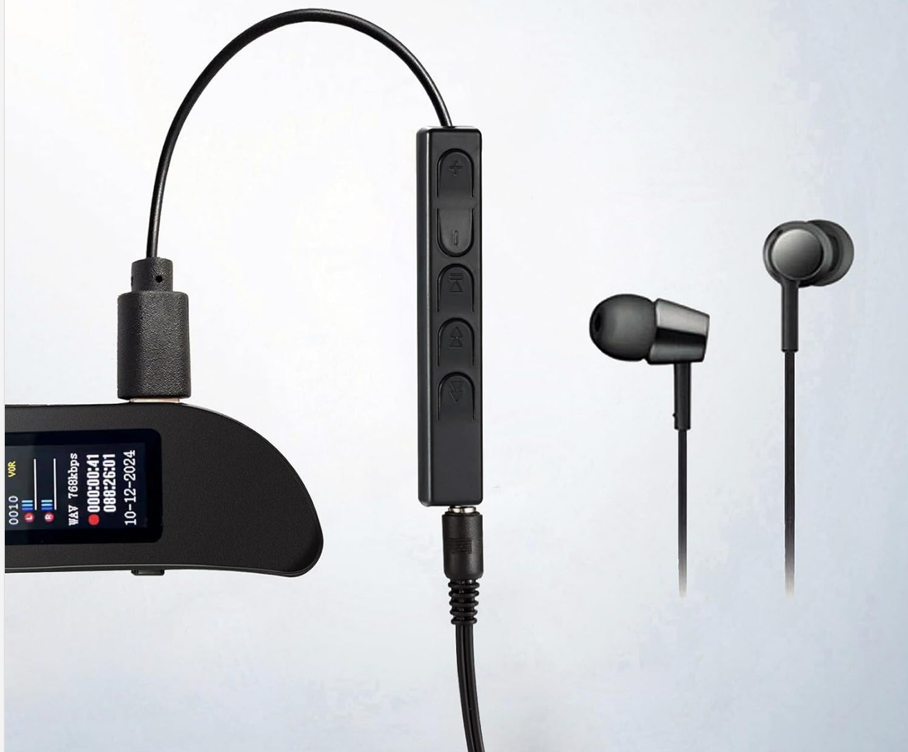
Image: The voice recorder connected to an external control unit and headphones, demonstrating playback without needing a computer.
