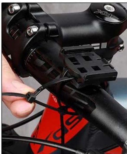
1. Attach the base to the handlebar
