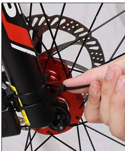
4. Attach wireless sensor by using warps
