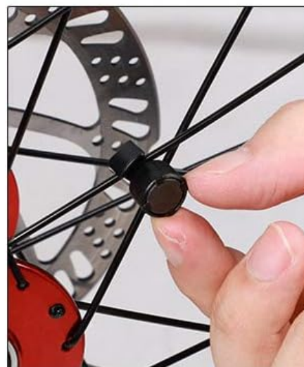
3. Attach the magnet to a spoke
