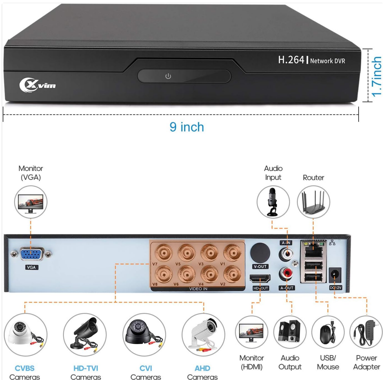
Image: Diagram of the DVR's back panel, showing ports for VGA, HDMI, video input (BNC), audio input/output, USB, and power.
