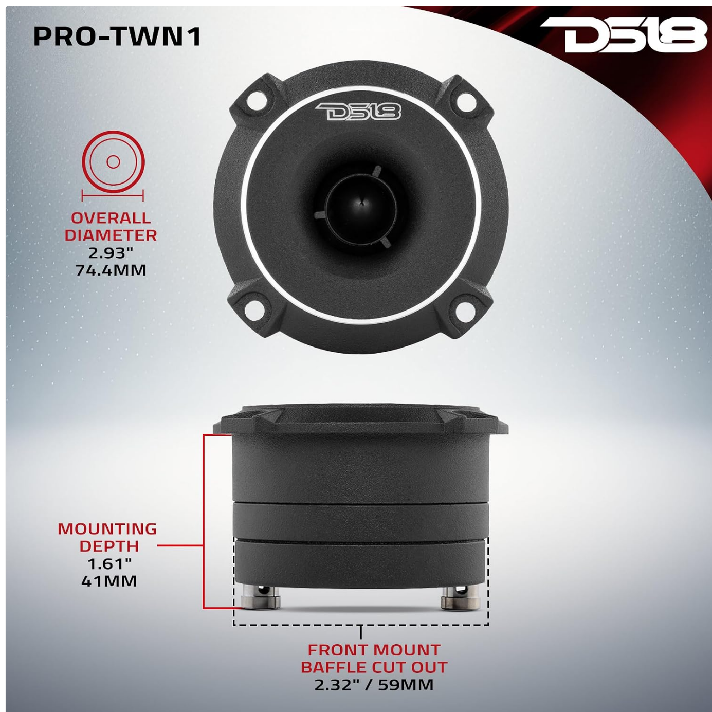
Figure 2.1: Tweeter dimensions for mounting. Overall Diameter: 2.93 inches (74.4mm), Mounting Depth: 1.61 inches (41mm), Front Mount Baffle Cut Out: 2.32 inches (59mm).
