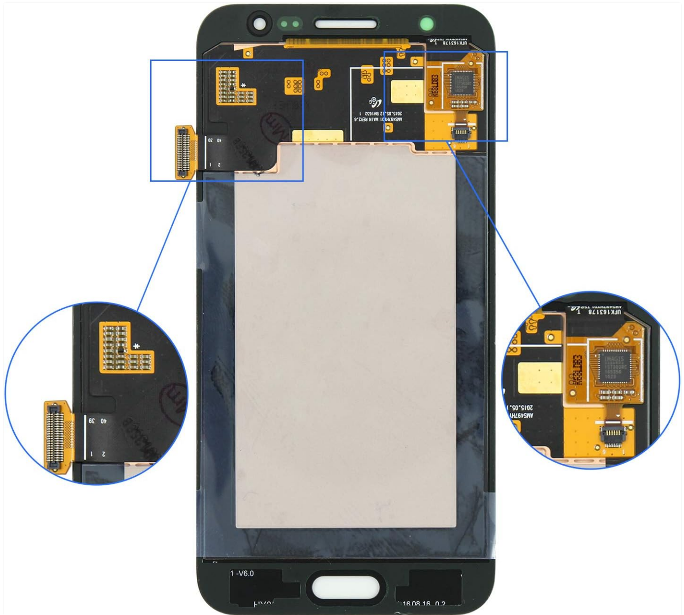
Image 4.1: Rear view of the AMOLED screen assembly, highlighting the flex cable connectors that attach to the phone's motherboard.
