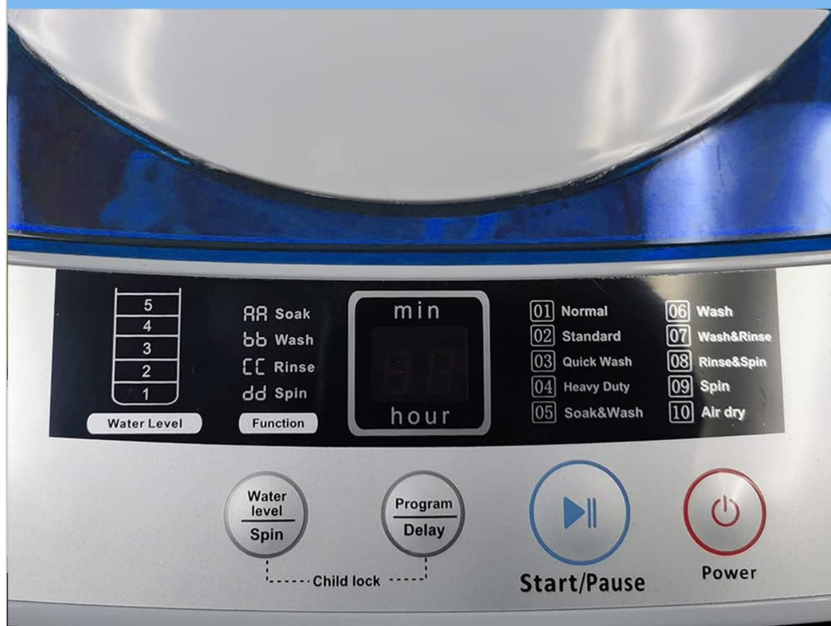
Image 3.1: Close-up of the Panda PAN356HB control panel. This image shows the buttons for Water Level, Function, Program, Delay, Start/Pause, and Power, along with the LED display and indicators for 10 wash programs and 5 water levels.
