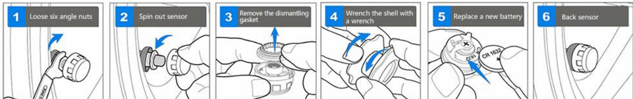
Image 5.1: External sensor battery replacement diagram.
